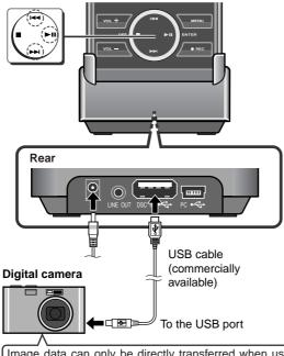
Image data can only be directly transferred when using the USB Mass Storage Class Bulk-Only Transport (BOT) recommended by Microsoft.
